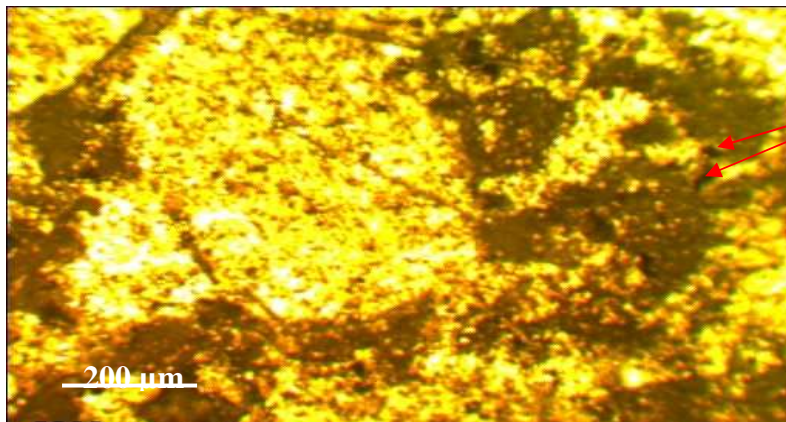
Figure 20. show the microstructure of Al – 5wt% Zn alloy after immersion, X 100
