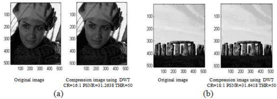
Figure 9: The original secret image and compression secret image with best compression (a) Lemas, (b) Stonehenge
