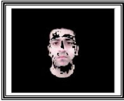
Figure (4) Face extraction and background removing to black color
