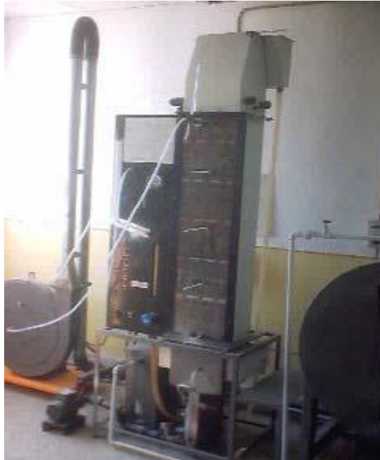
Figure (2) Schematic layout of Hilton forced draft water cooling tower
