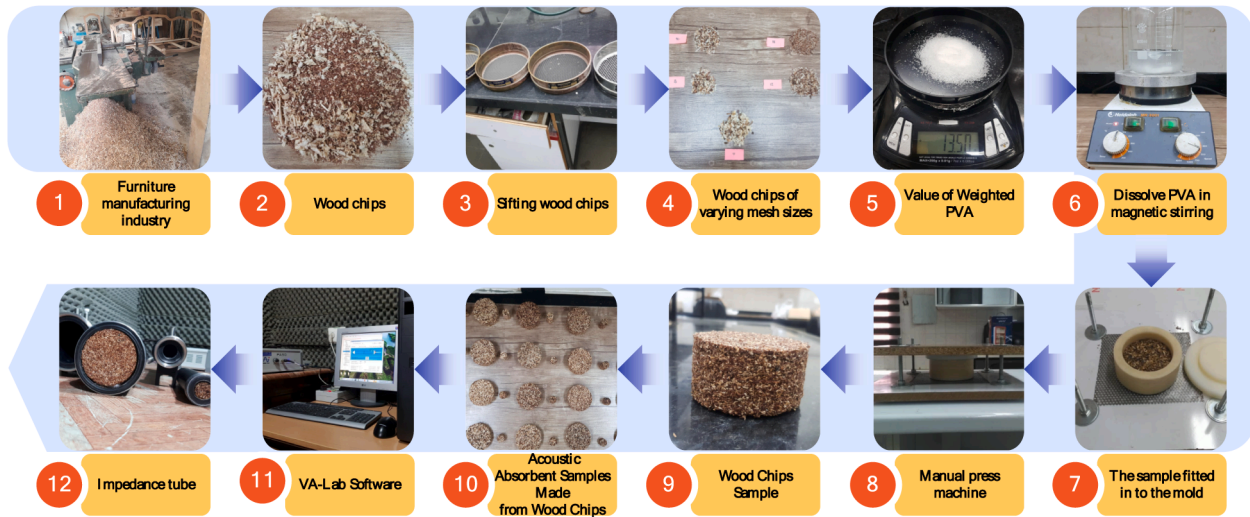
Fig. 1. Wood chips Sample preparation and acoustic absorption testing.
