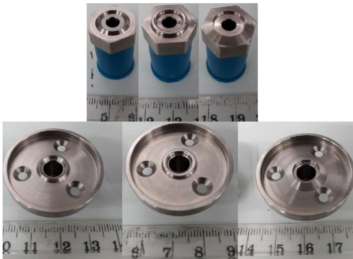
Figure 4. Knife-edge profiles used in the tests. Descending surface (top panel) is based on a modified 1/4" VCR blanking plug. L-R on both rows: 90°, VCR®, and CF®.
