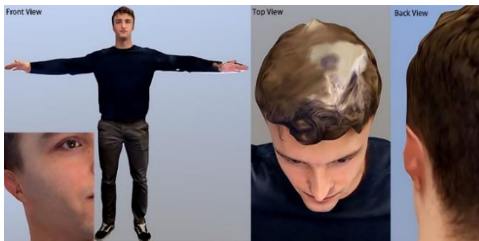
Figure 3.5. Artefacts and mesh distortion for the ears, when actor scanned in full body model (Huang, Twycross and Wild, 2019)
