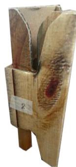
Figure 4.6. The connector for building the first floor
