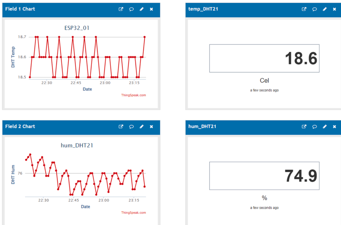
Fig. 18. ThingSpeak IoT platform interface of DHT21 sensor (25 Mar 2023).
