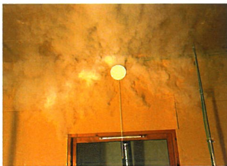
Figure 1. Development of the semi-radial wall jet from the ULA device.
