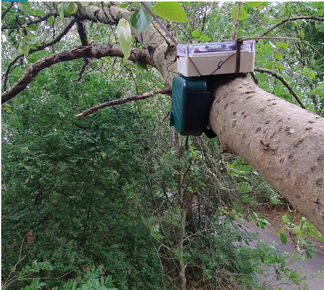
Figure 8: Bespoke open source hardware light logger deployed alongside AudioMoth audio logger to measure the impact of anthropogenic disturbance on bird and bat species. Image credit: Kristofer Chan, King's College London
