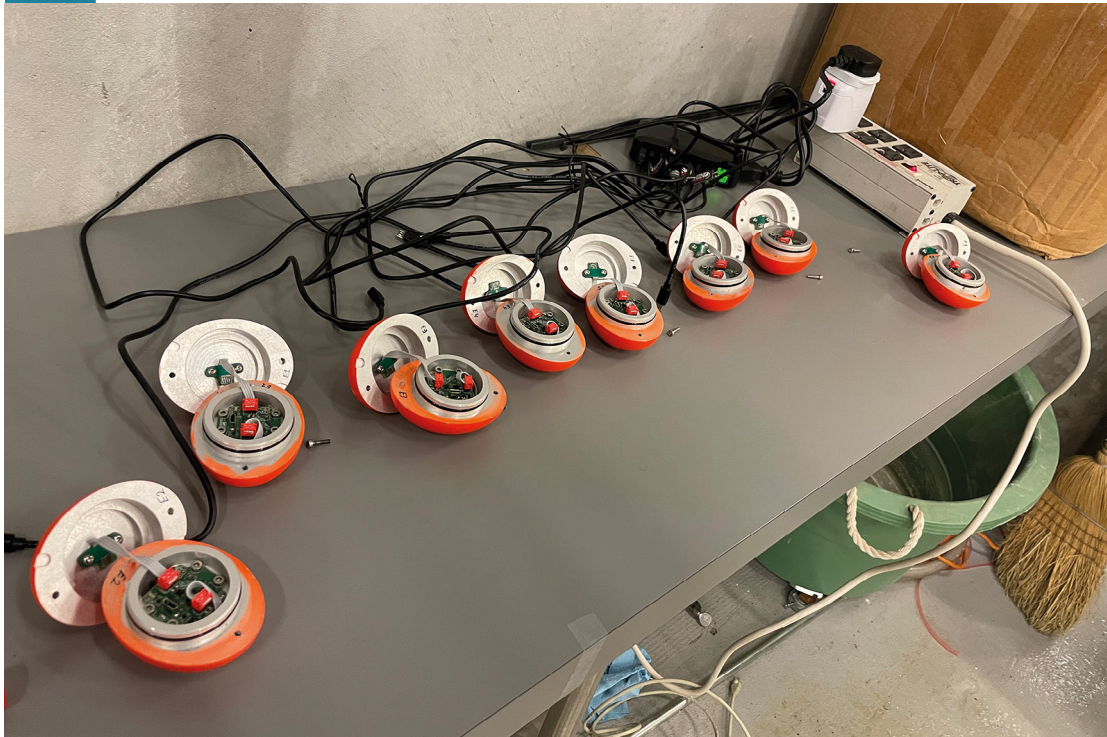
Figure 15: The new Kivi sensor, a “smart -pebble” designed to capture riverbed movements. xxiii Image credit: Georgios Maniatis, University of Brighton
