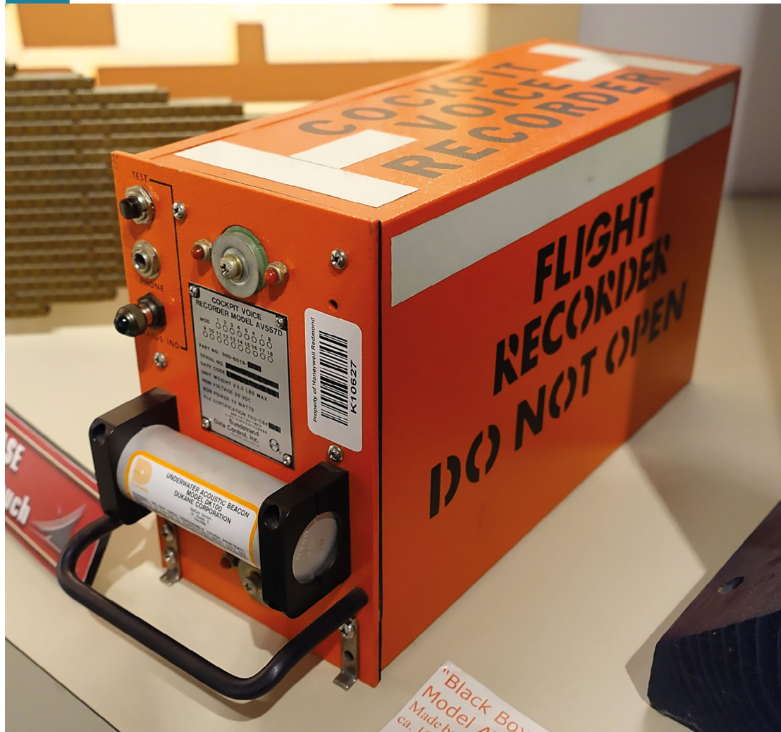
Figure 17: 'Black Box' flight recorder, challenging the idea of instrumentation adopting a 'black box' approach. Image credit: Wikimedia Commons
