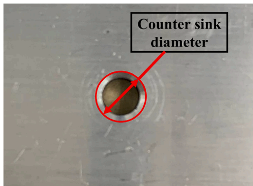
Fig. 16. The counter sink diameter measurement used to assess the precision of the deburring process.
