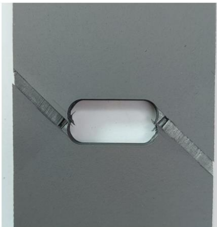
558 Figure 2: Photographs of 45° notch (top), -45° notch (middle) and 0° notch (bottom) specimens of the 559 geometry and type shown in Figure 1, following fatigue testing. As the -45° notch specimens were 560 monitored on their reverse side they have a similar appearance to the 45° notch specimens.
