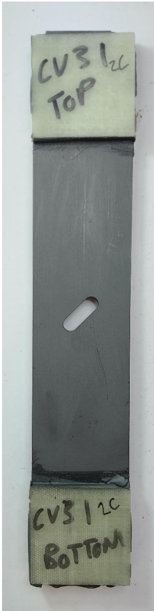
555 Figure 1: A typical 40 mm wide carbon-fibre composite laminate test-specimen with a 45° notch 556 machined at its centre and additional tabs bonded at each end.
