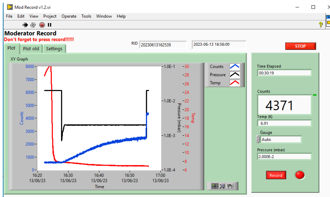
Figure 3.2: LabVIEW front panel for moderator growth. The temperature and pressure of the source chamber, and the counts are measured throughout and displayed.
