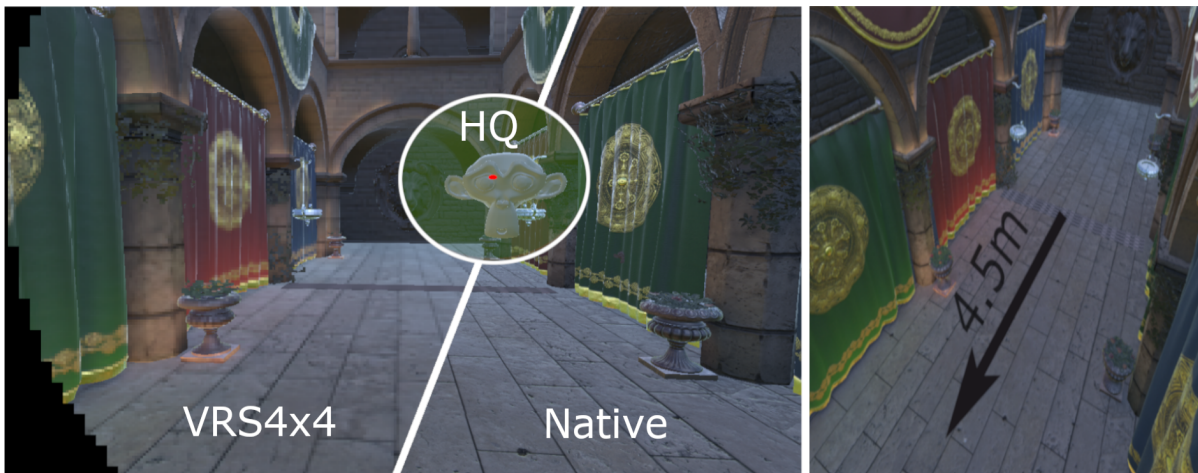
Figure 1: Left: representation of VRS4×4 shading reduction; in green the foveated region (HQ); the middle dot represents the eye-tracked focal point. The black margins show the algorithm culling everything outside the peripheral FOV. Towards right: a comparison to native shading (VRS1×1). Right: the path participants walked scaled to the dimension of the facility.
