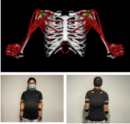
Fig. 2. Upper Limb Musculoskeletal Model; Participants were equipped with Xsens IMUs sensors for the demonstration.
