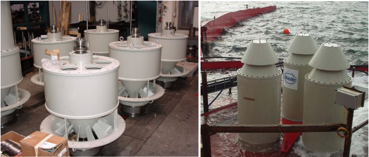
Figure 3. Left: The six axial propeller turbines being assembled at Kössler GmbH. Right: Turbines on board of the prototype in Nissum Bredning.
