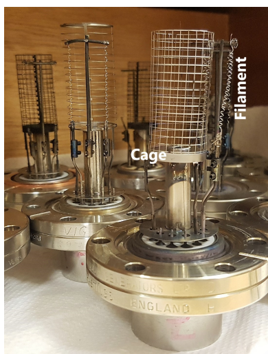
Figure 3.8: An ion gauge head.
