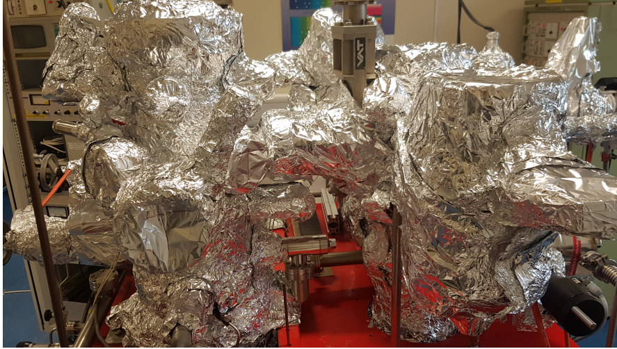
Figure 3.9: UHV chamber Madge during bakeout. The system is wrapped with heating tapes, and covered by aluminium foil.
