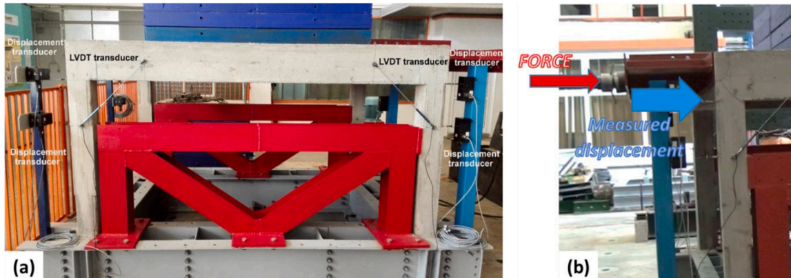
Fig. 3. (a) General test setup, and (b) actuator and stiff transfer plate to apply load.
