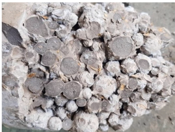
Fig. 22. Crushed pervious concrete.
