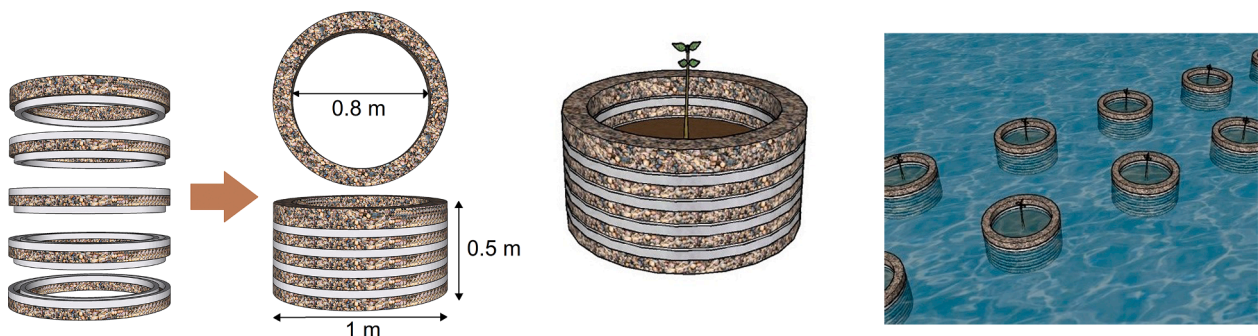
Fig. 1. Design of mangrove pot from pervious concrete.
