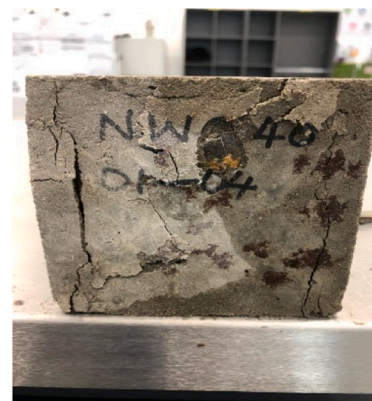
b. Normal concrete grade 40
