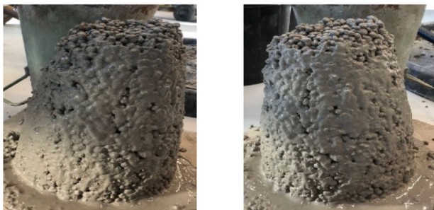
a: Concrete slump LC20/60 b: Concrete slump LC20/80
