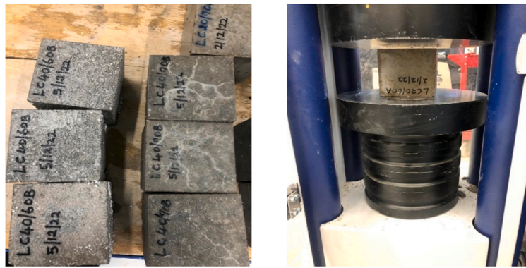
a. Samples for compressive test b. Sample under compressive test.
