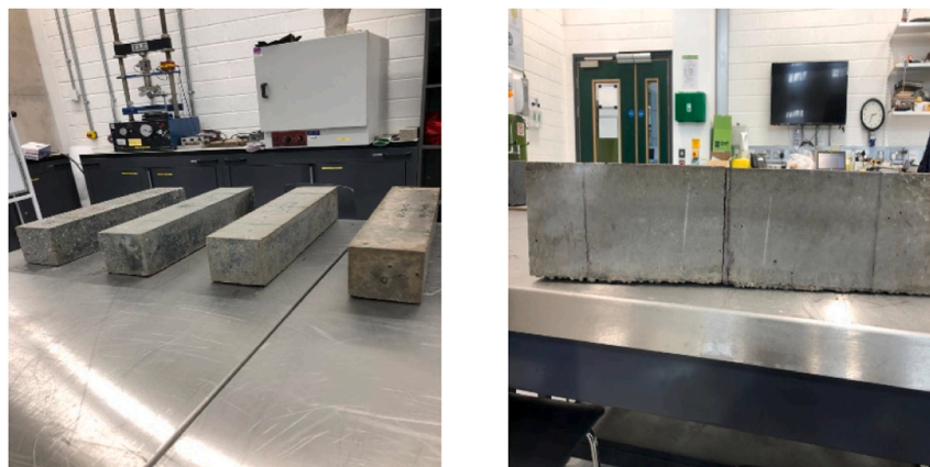
c. Set of Beam sample d. Sample failure under flexural
