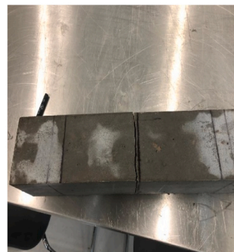
d. Flexural test failure
