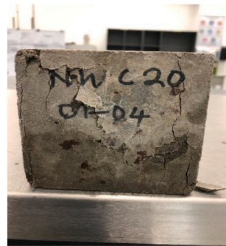
b. Normal concrete grade 20
