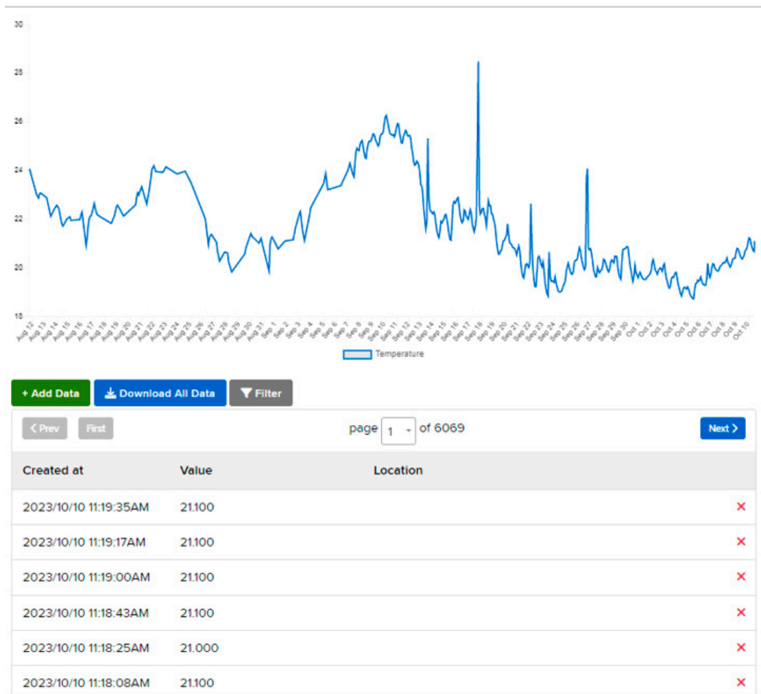
Figure 2. An example of a dashboard (user’s front end, above ) and a feed (developer’s back end, below ) on Adafruit IO.
