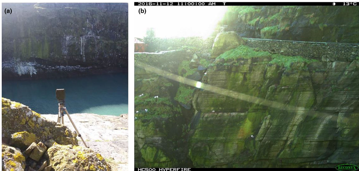
Figure 2. (a) Example time-lapse camera set-up on Skomer Island, Wales. This camera is mounted on a pre-made tripod typically used for spotting scopes, whereas other cameras are mounted on custom-built tripods made from scaffolding poles. Tripods are attached to the ground/nearby rock or weighed down with ballast. (b) Image taken at Skellig Michael, Ireland, in winter (12 November 2016), with Kittiwakes present on the cliffs.
