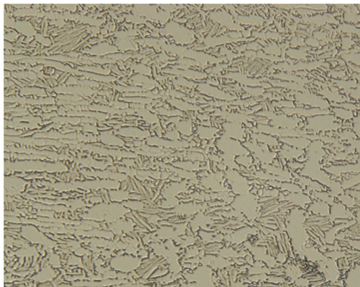
Fig. 8. Metallographic structure diagram of the machined surface layer material: (a) observed with the metallographic microscope, (b) obtained by the digital processing of metallographic diagram.
