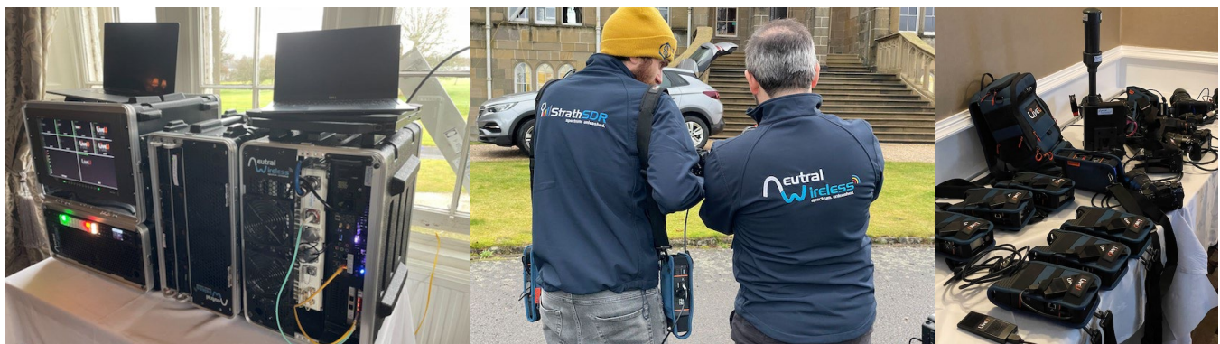
FIGURE 3: TESTING 20 1080P50 LRT STREAMS USING 12 LIVEU BONDED-CELLULAR DEVICES AT LOCH LOMOND.
