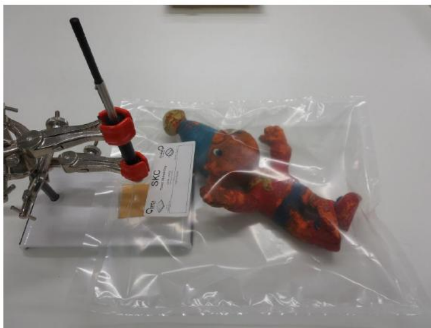
Figure 7. Non-destructive analysis of a PUR foam doll using a SPME fibre in a manual holder
