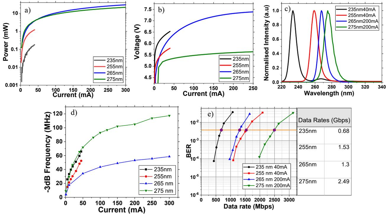
Figure 1 a) The LI b) IV c) spectra d) modulation bandwidth e) BER vs data rate for the 235nm, 255nm, 265nm and 275nm LEDs.
