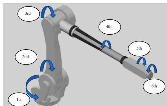
**Fig. 11.** Six axes' movements of the robotic welding.
