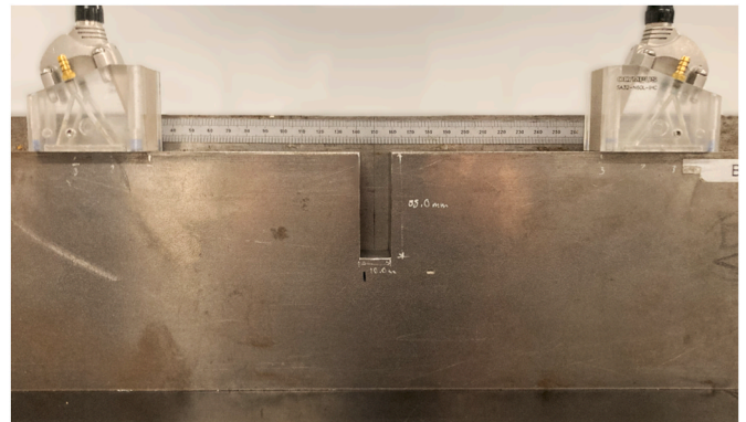
Fig. 2. Dual-tandem setup with two opposite-facing 5 MHz 64-element arrays mounted on 60LW Rexolite wedges.
