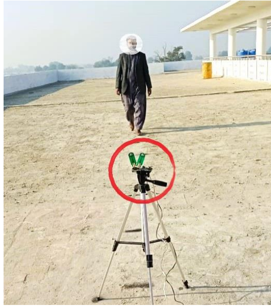
Figure 2: Subject moving toward UWB 410 radar mounted on stand and encircled red.
