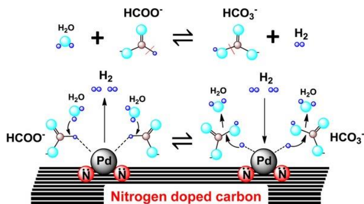
Figure 1.11. Mechanistic view of the bicarbonate – formate hydrogenation – dehydrogenation over the Pd/NMC. Reprinted from the reference [56] with the permission of the Wiley.
