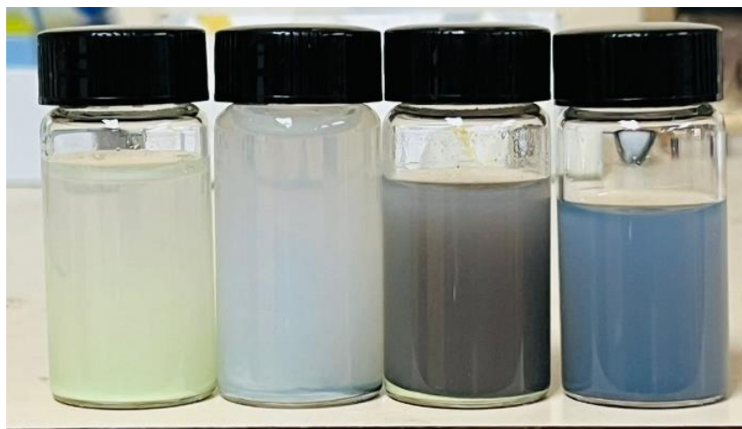
Figure 3.13. Evidence of H 2 spillover in liquid phase reactions. From left to right , (1): WO 3 + H 2 O, (2): WO 3 + H 2 O + H 2 , (3): WO 3 + H 2 O + Catalyst, and (4): WO 3 + H 2 O + Catalyst + H 2 .
