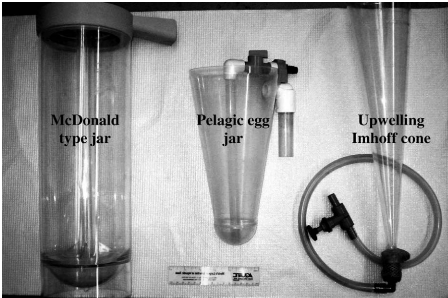
FIGURE 1.—Photograph of three incubator types used in a comparison of burbot egg and embryo survival.
