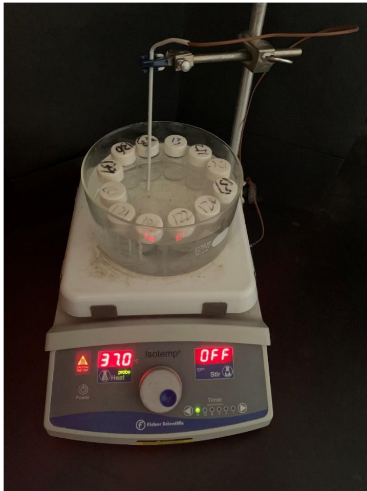
Figure 3.7: The apparatus for the immersion test.
