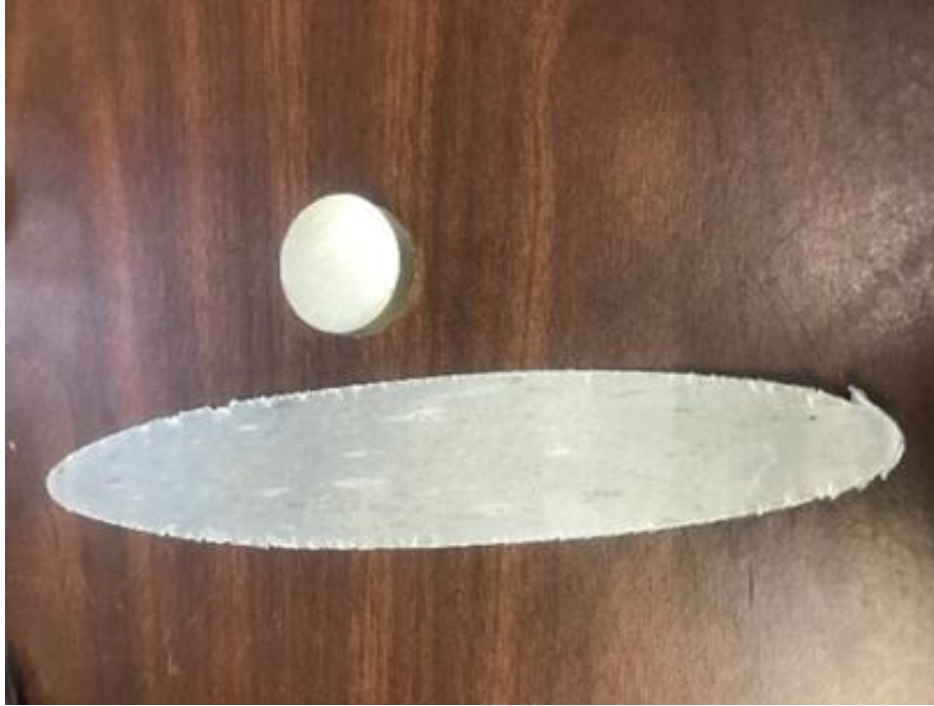
Figure 3.3: Mg block and Mg sheet before and after the rolling process.
