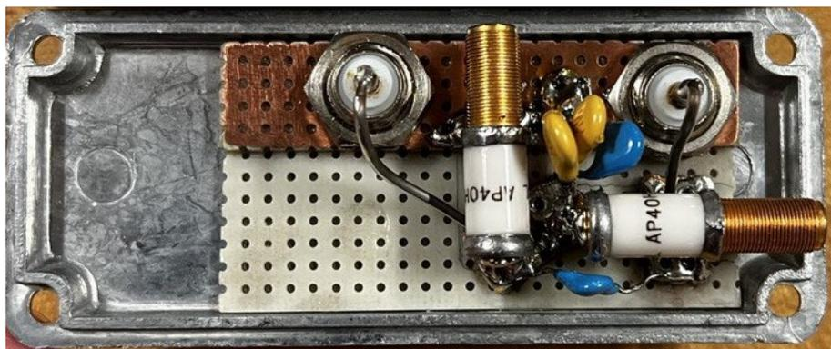
**Figure 3.10:** Tuning circuit: to tune the EPR coil to resonate at the alkali-metal hyperfine frequency and to be impedance matched with the amplifier.
