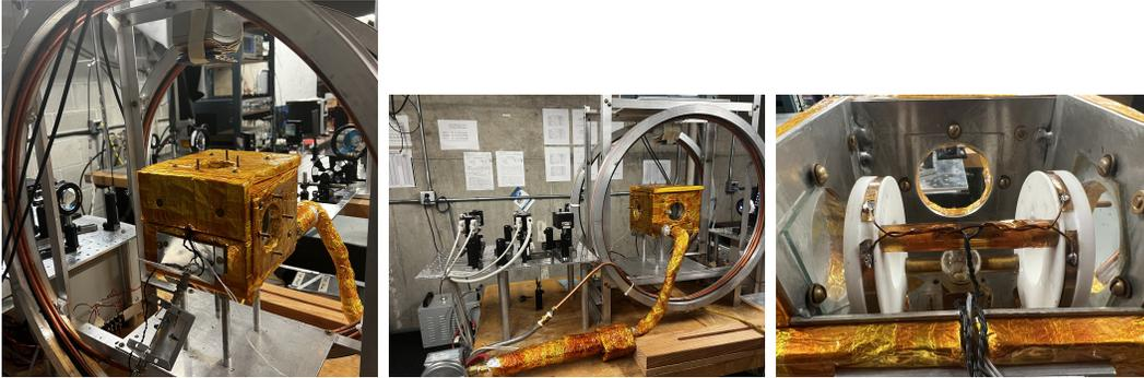
**Figure 3.8:** spin-exchange oven.
