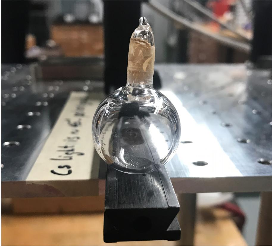
**Figure 3.6:** Sample cell containing alkali-metal and desired gases.
