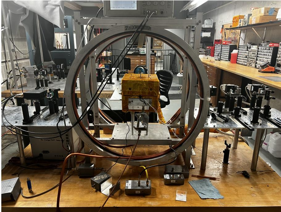
**Figure 3.9:** Helmholtz coils producing the static magnetic field  $B_0 \sim 28$  G and  $B_0 \sim 46$  G, being water cooled using copper tubes and room-temperature chiller.
