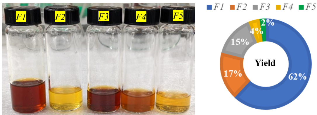
Figure 5.2: Yield of the sugar sub-fractions obtained from silica gel chromatography (left figure is the sugar sub-fractions dissolved in MeOH).
