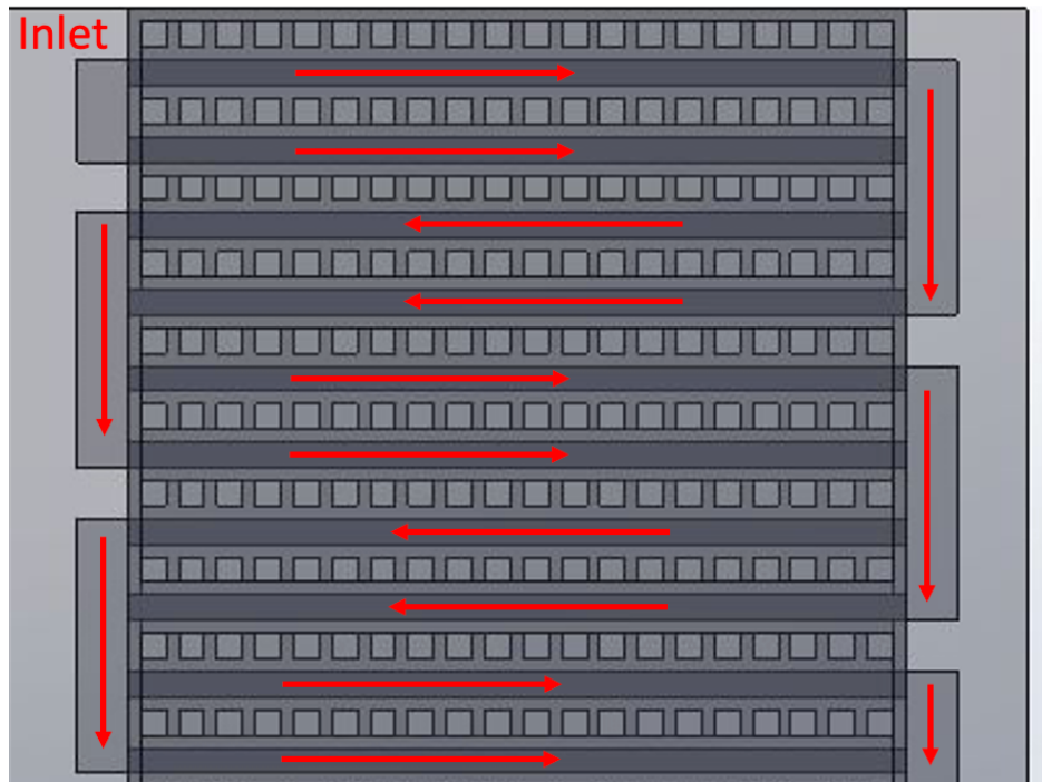
Figure 27 Gas Routing Highlighting Two Layers per Pass using an External Manifold; 0.05 mm Channel Dimensions with Vertical Multi-Pass System
