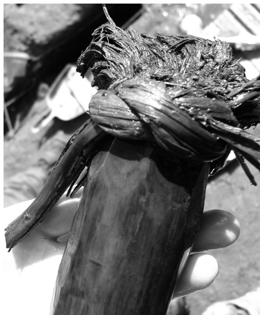
Figure 4.3 Wooden wedge, close up of rope collar to keep wedge from splitting while pounding – note the heavy wear from driving.
