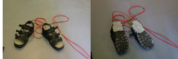
Figure 1: The shoe controller developed for the experiments.
