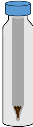
Figure 15. Schematic of sampling vial with insert used to collect the samples fossil plant material.
