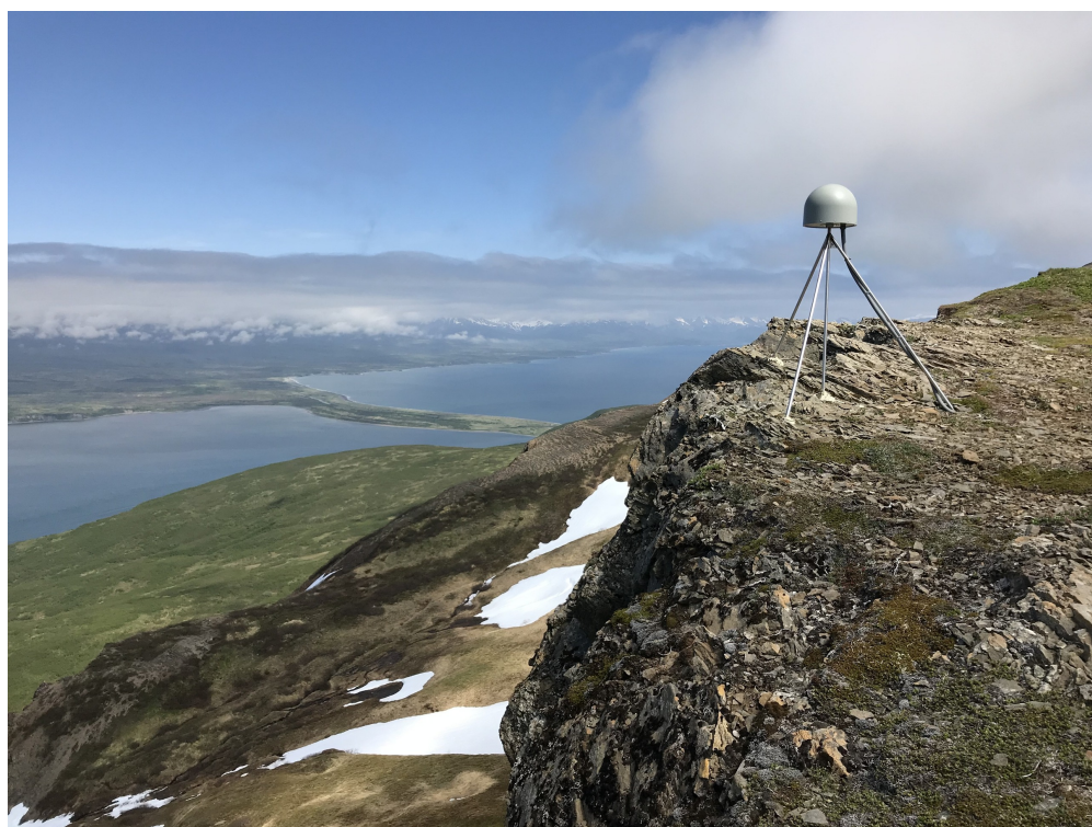
Figure 1.3: Station AB13 in Chignik, Alaska, an example of a permanent continuous GNSS station used in this study (credit: UNAVCO/Ellie Boyce)
