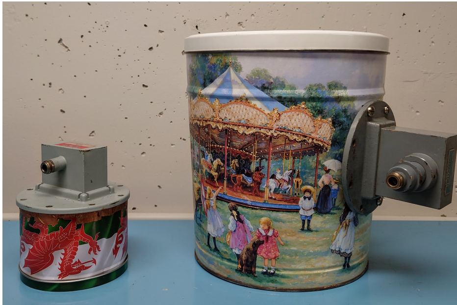
Figure 5.1: Photograph of the 1.4 L (left) and a scaled 5.2 L (right) cavities made of the tin-plated steel.
