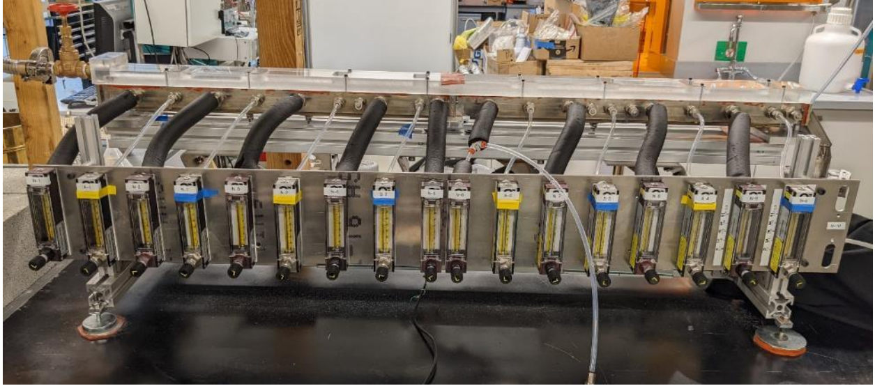
Figure 3.3. Experimental setup for powder convection tests. Powder travels through an acrylic chamber and over a porous baseplate during vibratory convection. Gas feed to the chamber is controlled by a series of rotameters
