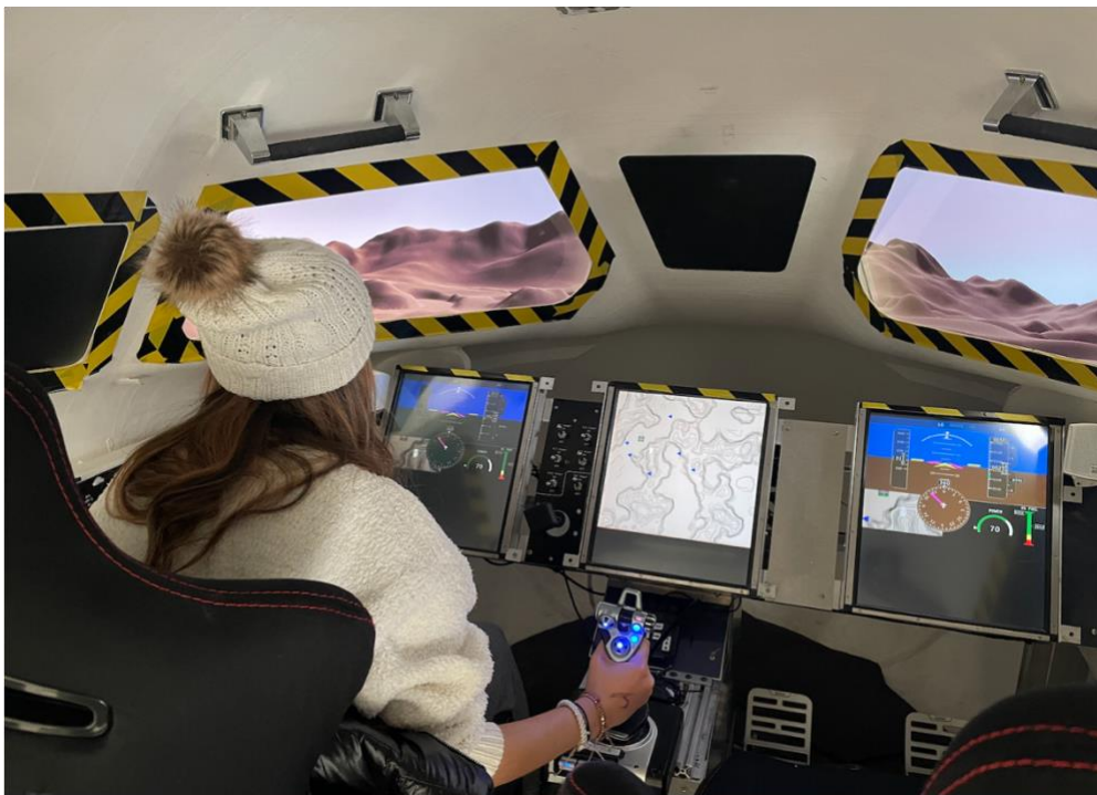
Figure 3.6: Subject performing EDL subtasks in AReS cockpit mock-up
