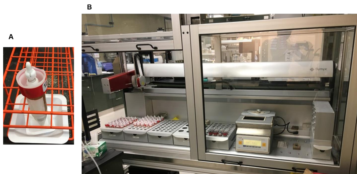
Figure C7. Images of A) a single hopper loaded with biomass B) The solids-loading robot with 70 biomass hoppers loaded.
