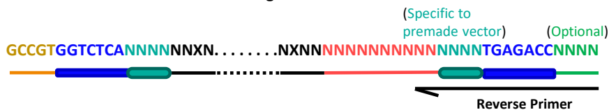
Figure B.3: Generalized design schematic of cassettes for Golden Gate-based cassette mutagenesis
