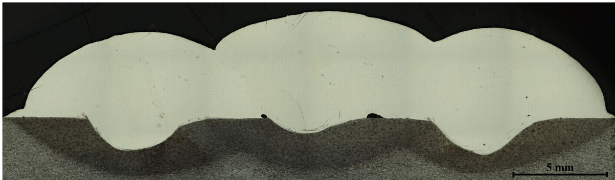
Figure 6: Cross-section of an ABA cladding with a distance between the 'A' weld beads of 18 mm
