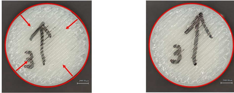
Figure 5: Visible roundness deviation in x-y direction for a) "Standard scaling", d = 15 cm (left) and b) "Adaptive Scaling V3.2", d = 35 cm (right)
