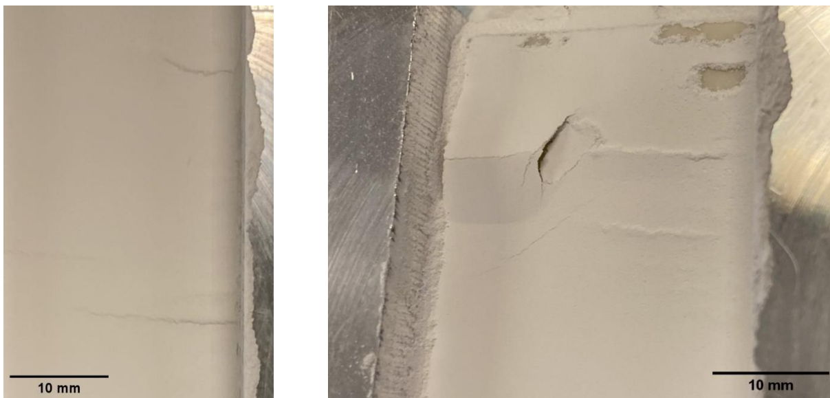
Figure 4: Visible cracks emanating from the edge of the compacted bed in Trial 4 (Left), Raised section of Trial 3 (Right). The effects of powder sticking to the roller are also apparent on the surface of the compacted powder on the right.
