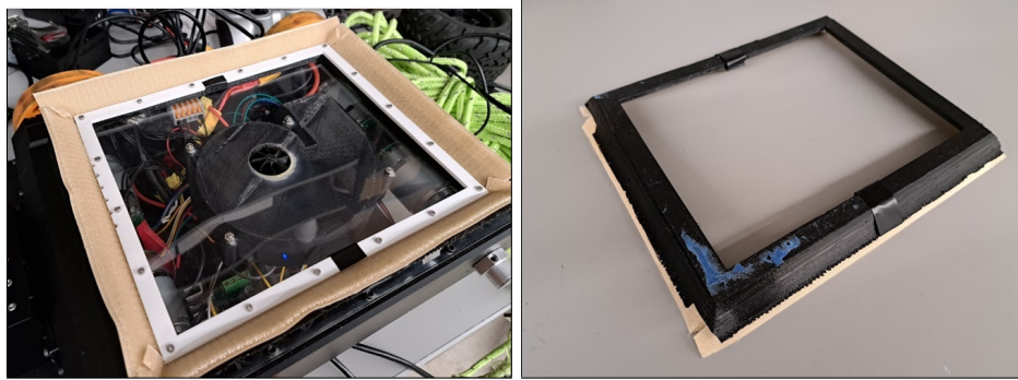
Figure 4.5: Flexible TPU skirt assembly.
