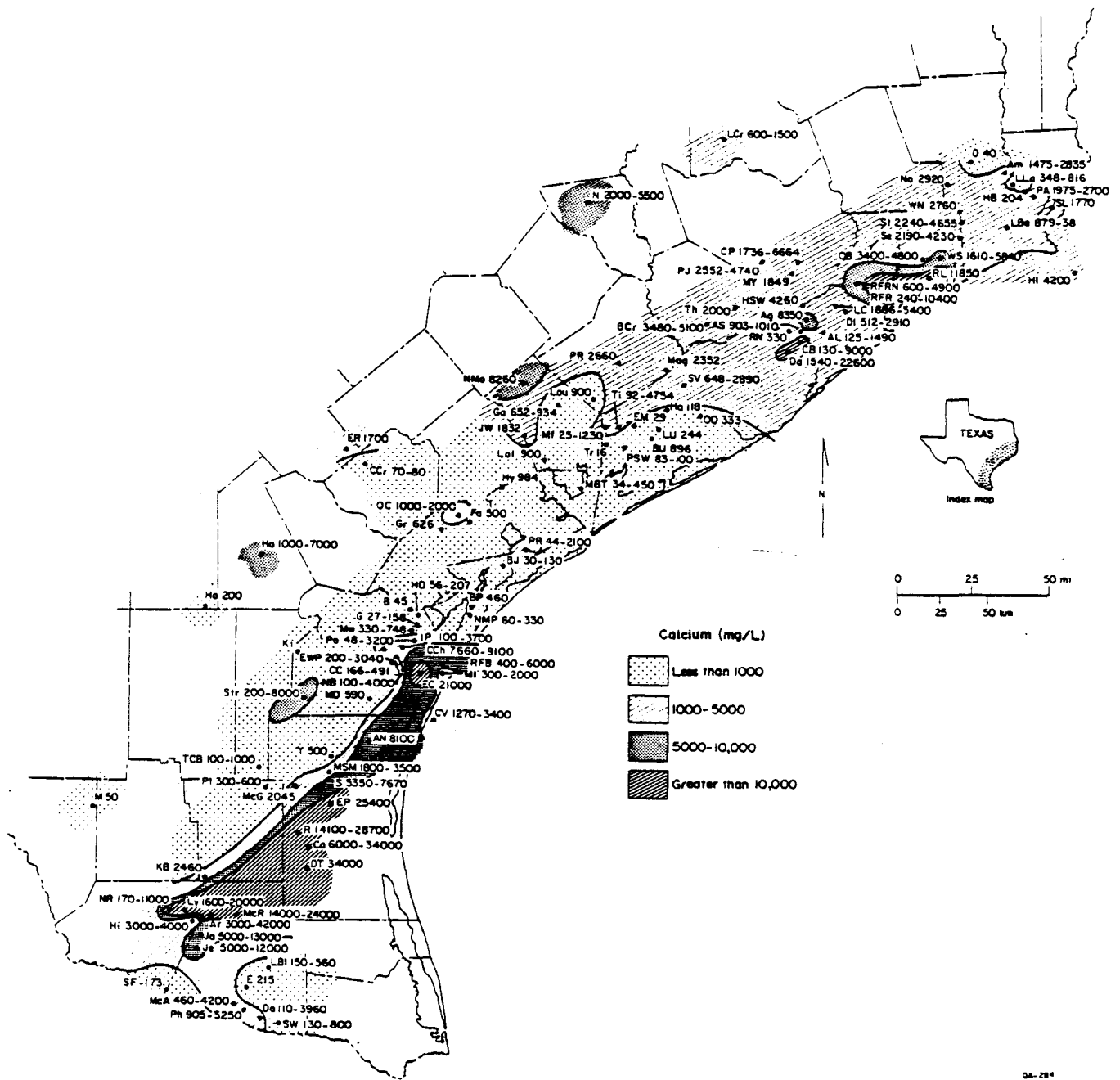
Figure II-30. Maximum concentrations of calcium in Tertiary formation waters. Chemical data from unpublished company files, Morton and others (1981), Kharaka and others (1977 and 1978), Jessen and Rolshausen (1944), and appendix II-A.
