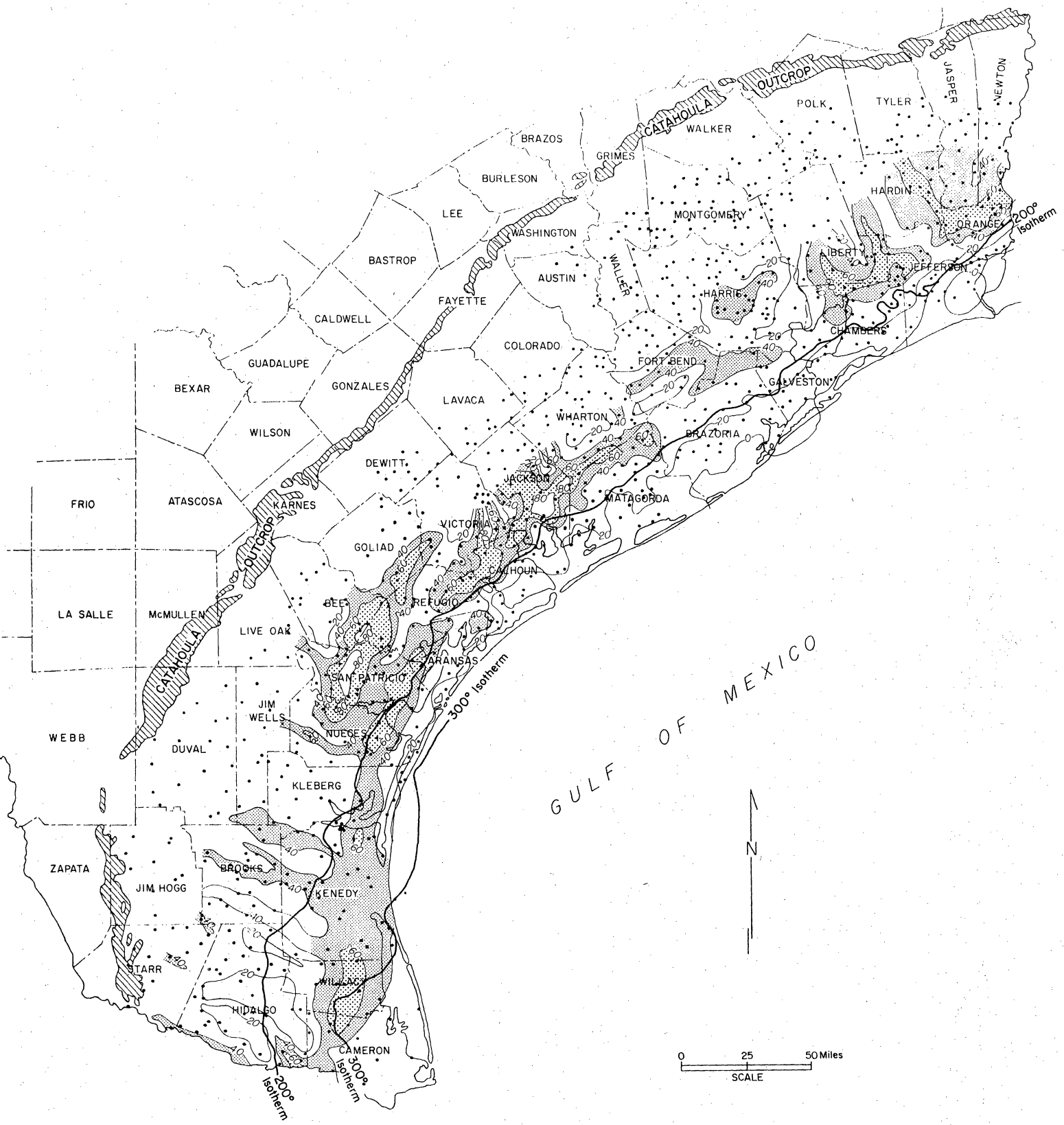
Figure 18. Sand percentage in unit T3-T4. The 200°F isotherm occurs within or just downdip of the main sand depocenter.
